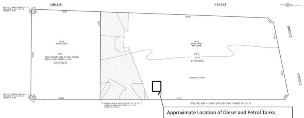
Figure 11 Location of Fuel Storage Tanks- Bridge and Alfred Block
